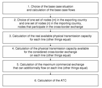
Fig. 1 Schema of ATC assessment process
