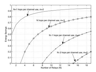
Fig. 1. The average energy savings curves versus the number of relays, using the distributed protocols for cooperative routing with distributed spacetime codes of m cooperating nodes when the end-to-end outage probability is  $\rho_{\rm max}=10^{-4}$ .
