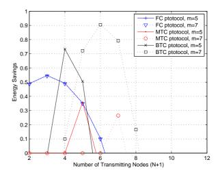
Fig. 2. The average energy savings curves versus the number of relays, using the distributed power allocation for cooperative routing with distributed space-time codes of m cooperating nodes when per hop outage probability requirement is  $\rho_0 = 10^{-5}$ .
