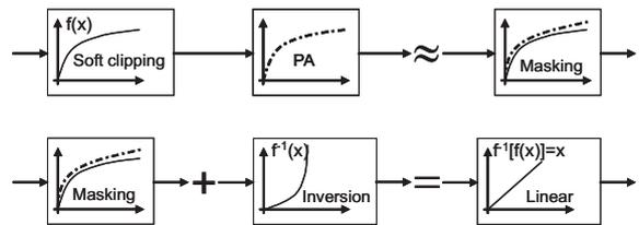
Fig. 2. PA masking and invertible clipping principle
