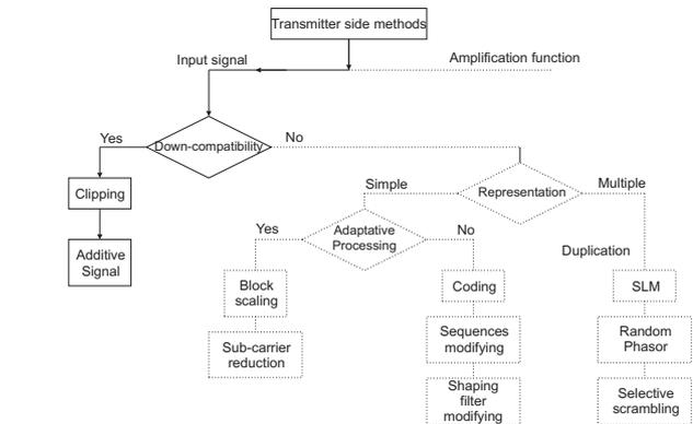
Fig. 1. Possible methods to carry out PAPR reduction
