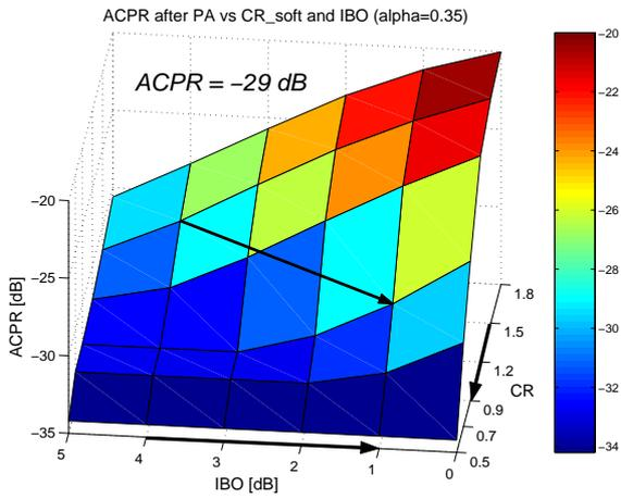
Fig. 6. Gain of 3 dB on the PA's IBO
