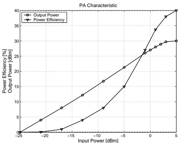
Fig. 11. Power amplifier characteristic (output power and efficiency)
