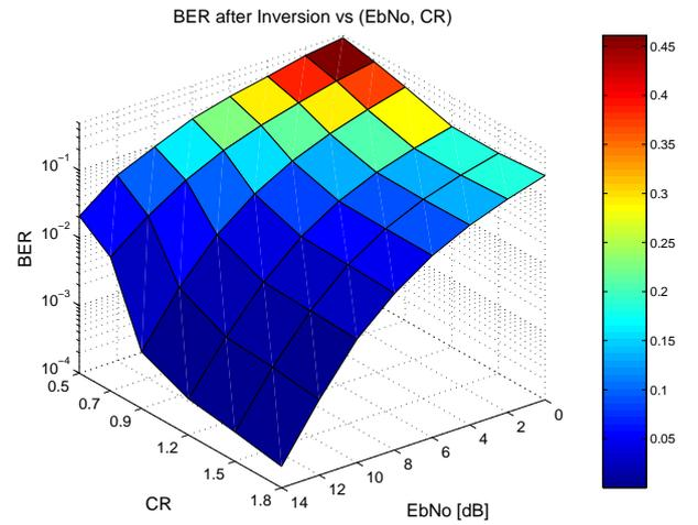
Fig. 8. BER after inversion on the noise channel
