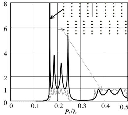
**Figure 27.** Coefficient  $|T_{2n}|$ , for  $n = 4$  and coefficient  $|t_8|$ .  $P_l = D = 2P_t$  and  $a/P_t = 5\%$ . The first peak of  $|T_{2n}|$  occurs at the same frequency that the first peak of  $|t_{2n}|$ .
