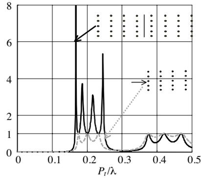
**Figure 26.** Coefficient  $|T_{2n}|$ , for  $n = 4$  and coefficient  $|t_4|$ .  $P_l = D = 2P_t$  and  $a/P_t = 5\%$ . In the first pass-band,  $|T_{2*4}|$  has two more peaks than  $|t_4|$ . In the second pass-band the two coefficients have the same number of peaks.
