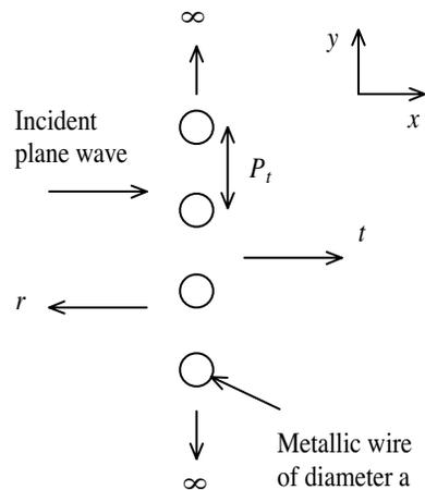
**Figure 1.** Partially Reflecting Surface of metallic wires.
