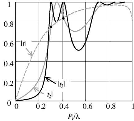
**Figure 18.** Coefficients  $|t|$ ,  $|t_2|$ , and  $|t_3|$ . The intersections between  $|t|$  and  $|t_2|$  correspond to the peaks of  $|t_3|$ . The minimum between two peaks of  $|t_3|$  is determined by  $|t|$ .
