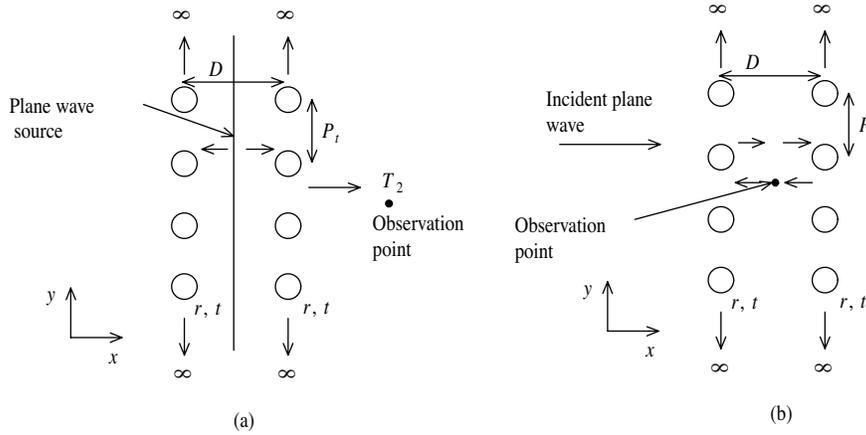
**Figure 22.** Two equivalent problems: (a) Fabry-Perot cavity excited by a plane wave source from its inside. Calculation of the total transmitted wave outside the cavity (b) Fabry-Perot cavity excited by a plane wave source from outside. Calculation of the wave inside the cavity.
