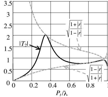
**Figure 25.** Coefficient  $|T_2|$ , envelopes of minima and maxima.
