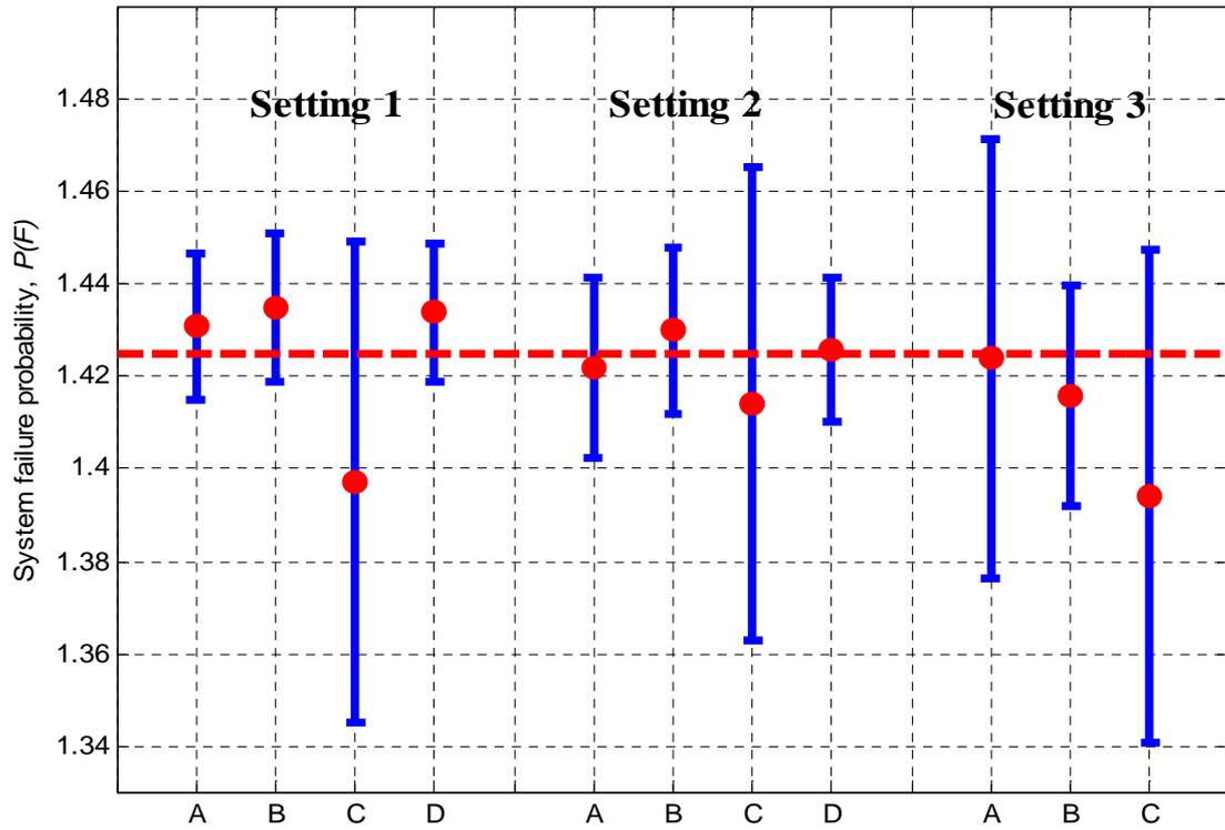
Figure 3. Point estimates  $\hat{P}(F)^{N_T}$  (dots) of the failure probability  $P(F)$  obtained with  $N_T = 10000$  samples in settings 1, 2 and 3 (Table 3) of Application 1 of Case study 1, along with the corresponding 95% CIs (bars) and the true (i.e., reference) value of the system failure probability  $P(F)$  (i.e.,  $P(F) = 1.425 \cdot 10^{-4}$ ) (dashed line)
