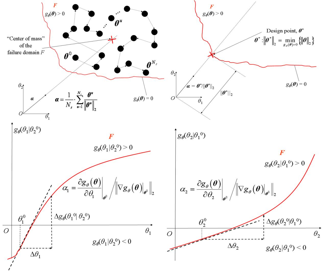
Figure 1. Methods for estimating the Line Sampling important unit vector  $\alpha$ . Top, left: normalized “center of mass” of the failure domain  $F$  in the standard normal space [25]; top, right: direction of the design point of the problem in the standard normal space [27], [36]; bottom, left and right: normalized gradient of the PF  $g_{\theta}(\cdot)$  evaluated at a selected point  $\theta^0$  (e.g., the nominal point) in the standard normal space [26]
