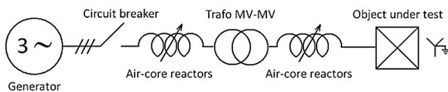
Figure 5: Overview of the Medium Voltage test network.
