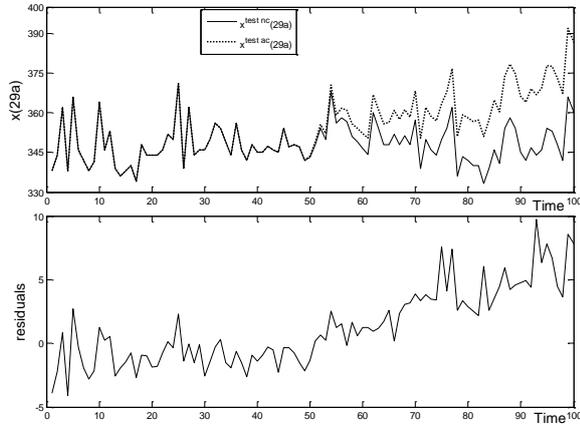
Figure 7. Top: time evolution of the first seal flow,  $x^{test-nc}(29a)$ , during 100 consecutive hours in normal condition (continuous line) and its evolution,  $x^{test-ac}(29a)$ , when a deterioration of the RCP seal is simulated (dotted line). Bottom: residuals between the measured signal,  $x^{test-ac}(29a)$ , and its reconstruction  $\hat{x}_{nc}^{test-ac}(29a)$ .
