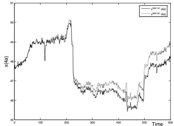
Fig. 3. Temperature of the water flowing to the first seal of the pump in line 1,  $x^{test-nc}(4a)$ , during 600 consecutive hours (continuous line) and its measurement obtained by a drifted sensor,  $x^{test-ac}(4a)$  (dotted line).
