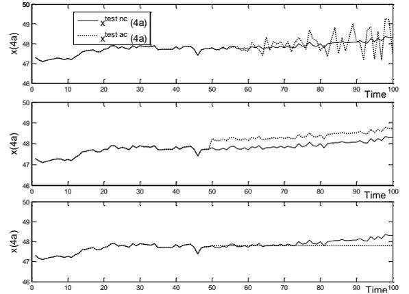
Fig. 5. Three different sensor failures: measurement noise increase (top), sensor offset (middle), sensor stuck (bottom).
