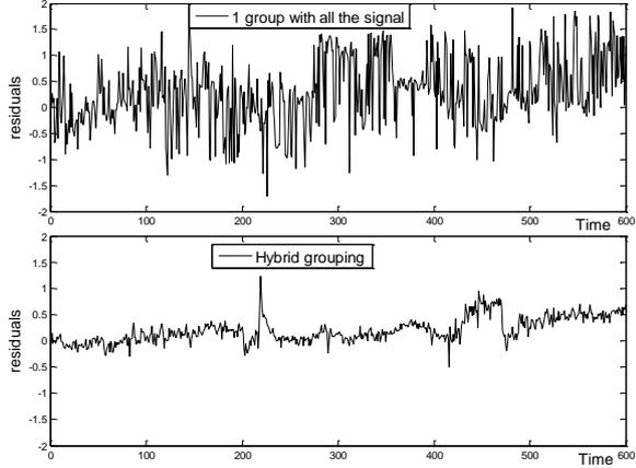
Fig. 4. residuals between the measured signal by the faulty sensor,  $x^{test-ac}(4a)$ , and its reconstruction  $\hat{x}_{nc}^{test-ac}(4a)$  when a single group formed by all signals (top) and the hybrid grouping (bottom) are used for the signal reconstruction.
