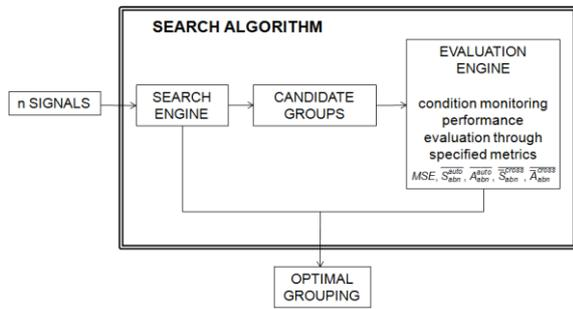
Fig. 1. Wrapper approach for optimal signal grouping.
