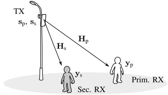
Fig. 1. Layout for simultaneous primary and secondary transmissions.
