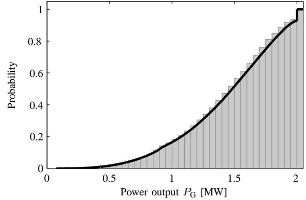
Fig. 5. Distribution function of the power output  $P_G$ , for a mean wind speed  $\bar{v} = 12 \text{ m/s}$ : result obtained with the generalized FPE (full line), compared to a reference Monte-Carlo simulation (cumulative histogram).
