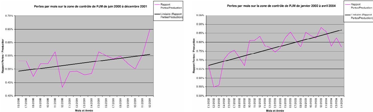
Figure 6 Evolution trends of EHV network losses vis-à-vis energy generation on the PJM control area from June 2000 to December 2001 and from January 2002 to April 2004 (own calculus from PJM data)
