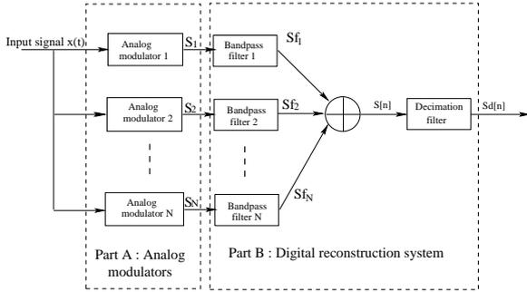
Figure 2: Wide band converter's architecture
