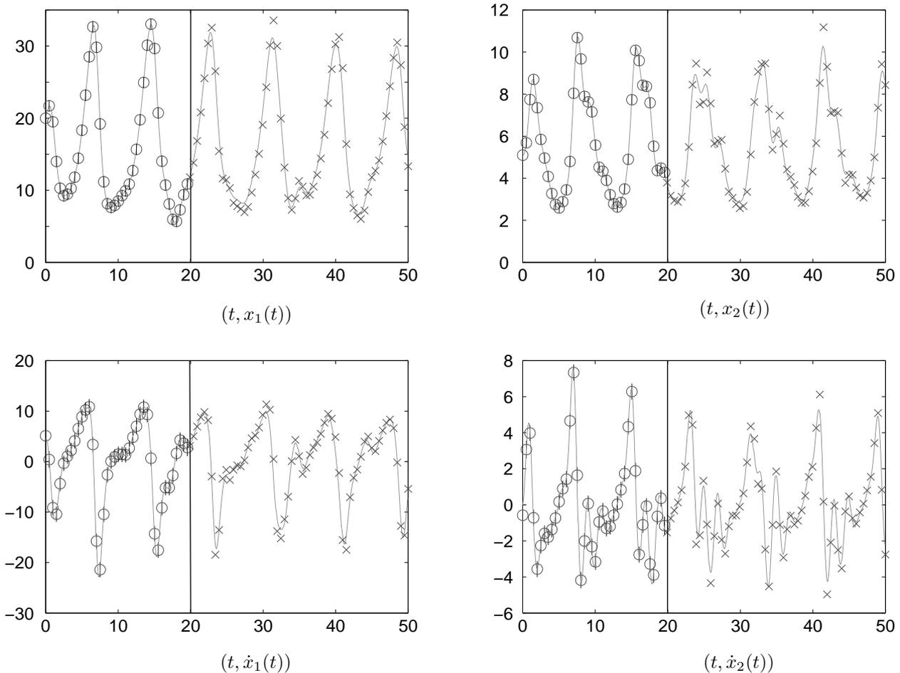
Figure 2. Simulation of the system (20). Solid line:  $x_1(t)$ ,  $x_2(t)$ ,  $\dot{x}_1(t)$  and  $\dot{x}_2(t)$  computed by the ODE solver. Circles: the observations and the estimated derivatives in the identification procedure. Crosses: components of the state vector and their derivative obtained with the proposed simulation method. The vertical line at  $t = 20$  marks the starting time of the simulation.
