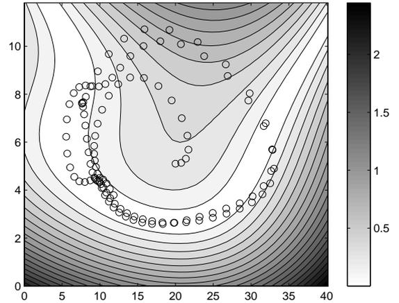
Figure 4. Contour plot in the plane  $(x_1, x_2)$  of the absolute difference between  $f_1(x_1, x_2, 0)$  and its approximation  $\widehat{f}_1(x_1, x_2, 0)$  obtained by our identification procedure. The circles indicate the position of the observations in the plane  $(x_1, x_2)$ .
