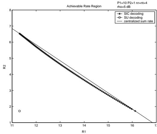
Figure 2: Achievable rate pairs for the **temporal** power allocation case for  $P_1 = 10$ ,  $P_2 = 1$ ,  $n_r = n_t = 4$ ,  $\rho = 5dB$ . The performance of the decentralized MAC with coordination is close to that of its centralized counterpart.
