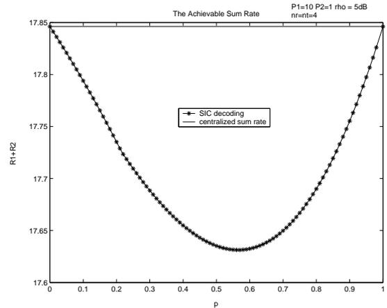
Figure 1: Temporal power allocation case. MAC sum-rate versus  $p$  for  $P_1 = 10$ ,  $P_2 = 1$ ,  $n_r = n_t = 4$ ,  $\rho = 5$  dB. The sum-rate of fading MIMO MACs is almost reached whatever the coordination signal distribution.
