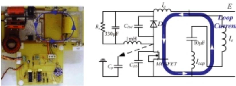
Figure 10. The radiating loop current in the DUT.
