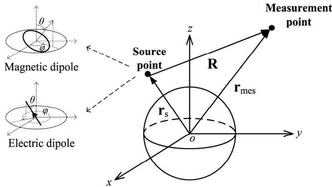
**Figure 1.** The definitions of equivalent radiating dipoles.
