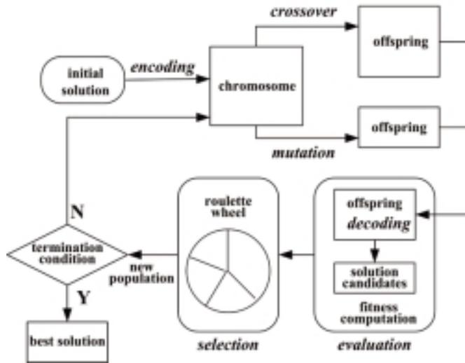
Figure 2. The general structure of standard genetic algorithm.
