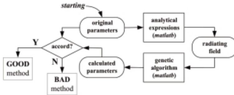
**Figure 4.** The flow of validation by analytical results.
