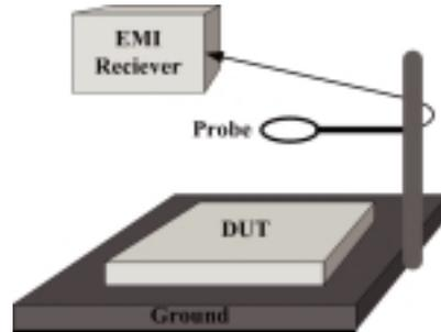
**Figure 7.** The configuration of the test bench.
