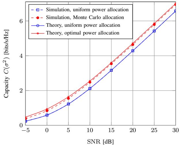
Fig. 2. Uplink capacity of a  $K = 3$ -clustered orthogonal CDMA, uniform and optimal power allocation,  $N = 8$ . For user  $n$  in cluster  $k$ ,  $\lambda_{kn} = -\alpha_k(n-1)/(N-1)$  dB,  $\alpha_1 = 10$  dB,  $\alpha_2 = 20$  dB,  $\alpha_3 = 30$  dB.
