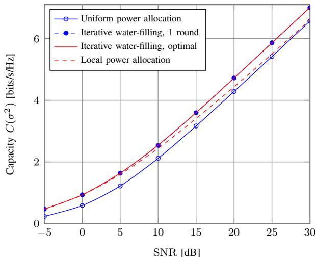
Fig. 3. Uplink capacity of a  $K = 3$ -cluster orthogonal CDMA, iterative water-filling power allocation,  $N = 8$ . For user  $n$  in cluster  $k$ ,  $\lambda_{kn} = -\alpha_k([n-1]/[N-1])$  dB,  $\alpha_1 = 10$  dB,  $\alpha_2 = 20$  dB,  $\alpha_3 = 30$  dB.
