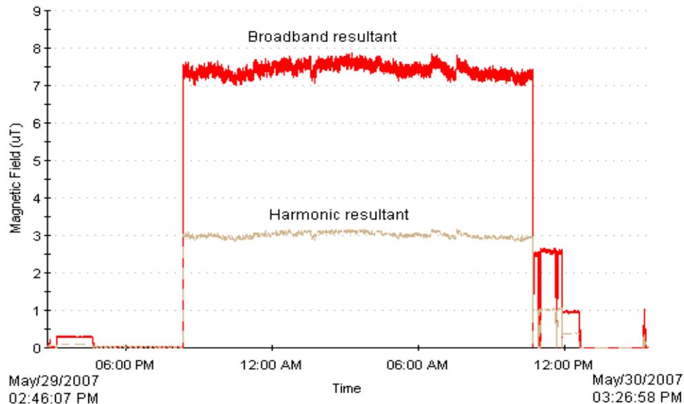
Fig.3: Example of a MF series which an important part was generated by a clock radio.
