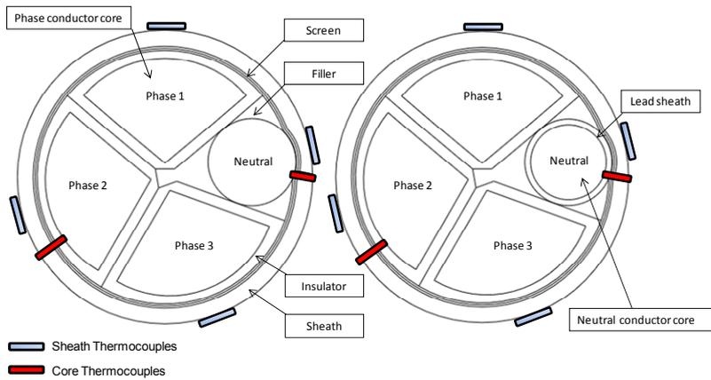
Fig. 1 . Cable geometry and thermocouple position
