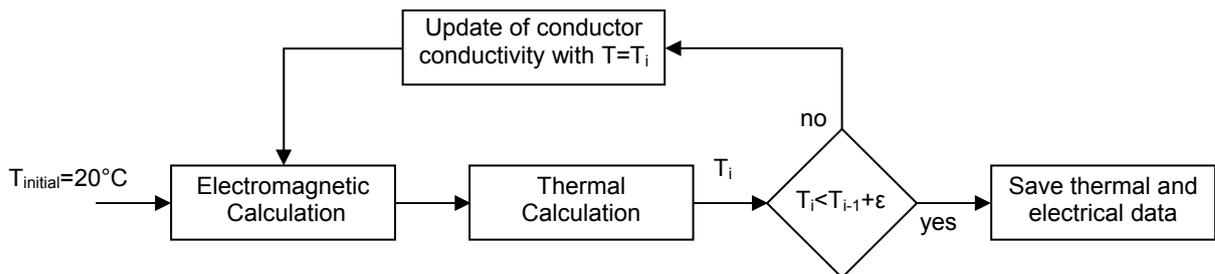
Fig. 4 Simulation process
