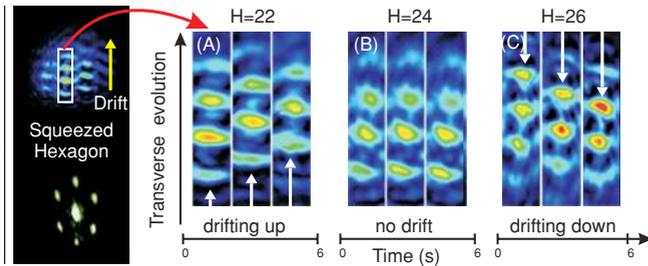
FIG. 4. (Color online) Time evolution of the transverse profile of the squeezed hexagon from Fig. 2(C). From left to right, drifting pattern passing from a positive transverse phase velocity  $v \simeq +\pi/3$  rad  $s^{-1}$  (A) to null (B) then to a negative value  $v \simeq -\pi/3$  rad  $s^{-1}$  (C) for different  $H$ .
