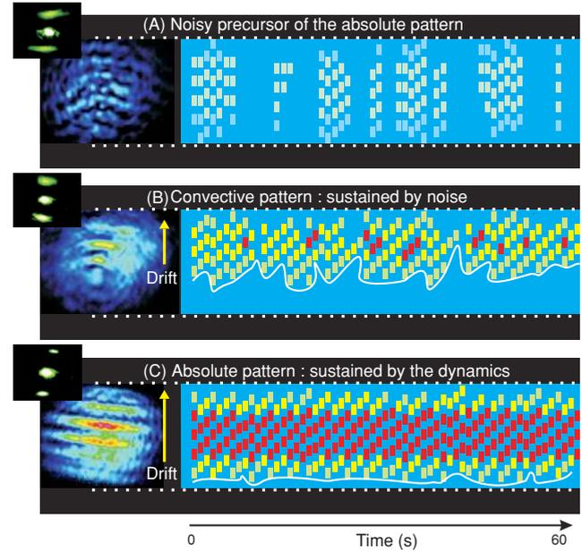
FIG. 5. (Color online) Spatiotemporal evolution of the transverse profile of the stripe pattern obtained in Fig. 2(B) ( $H = 10 \mu\text{m}$ ) for different powers of the pump beam: (A) 15 mW, (B) 30 mW, (C) 55 mW. The dotted lines depict the available space for the growing process of the pattern. From blue to red, the colors indicate respectively an evolution from low to high intensities in the near-field pattern. (Inset) Corresponding far field.
