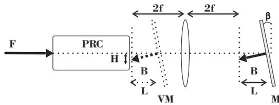
FIG. 1. Schematic of the setup composed of a photorefractive crystal (PRC) in a single-feedback configuration. M, mirror; VM, virtual mirror; L, distance between the virtual mirror and the crystal;  $\beta$ , mirror tilt angle;  $H = L \sin \beta$ , transverse shift (in  $\mu\text{m}$ ); F and B correspond respectively to the forward and backward beams responsible for the pattern formation.
