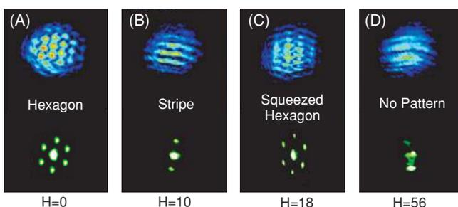
FIG. 2. (Color online) Different patterns obtained for different transverse shifts  $H$  (in  $\mu\text{m}$ ) and for a virtual mirror located outside the crystal ( $L \approx 1$  mm). The pump beam intensity is fixed to the value  $I_p \approx 45$  mW. Top, near field; bottom, far field.
