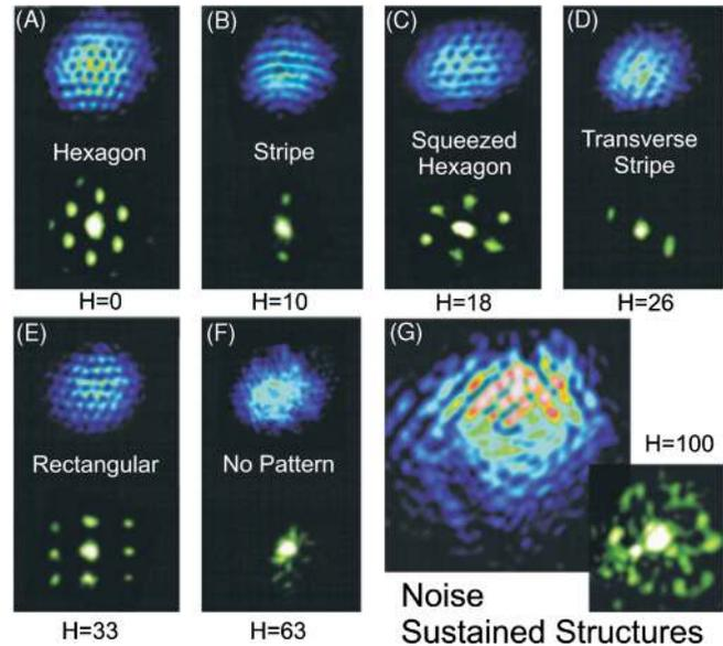
FIG. 3. (Color online) Different patterns obtained for different transverse shifts  $H$  (in  $\mu\text{m}$ ) and for a virtual mirror located inside the crystal ( $L \approx -2$  mm). The pump beam intensity is fixed to the value  $I_p \approx 45$  mW. Top, near-field; bottom, far-field.
