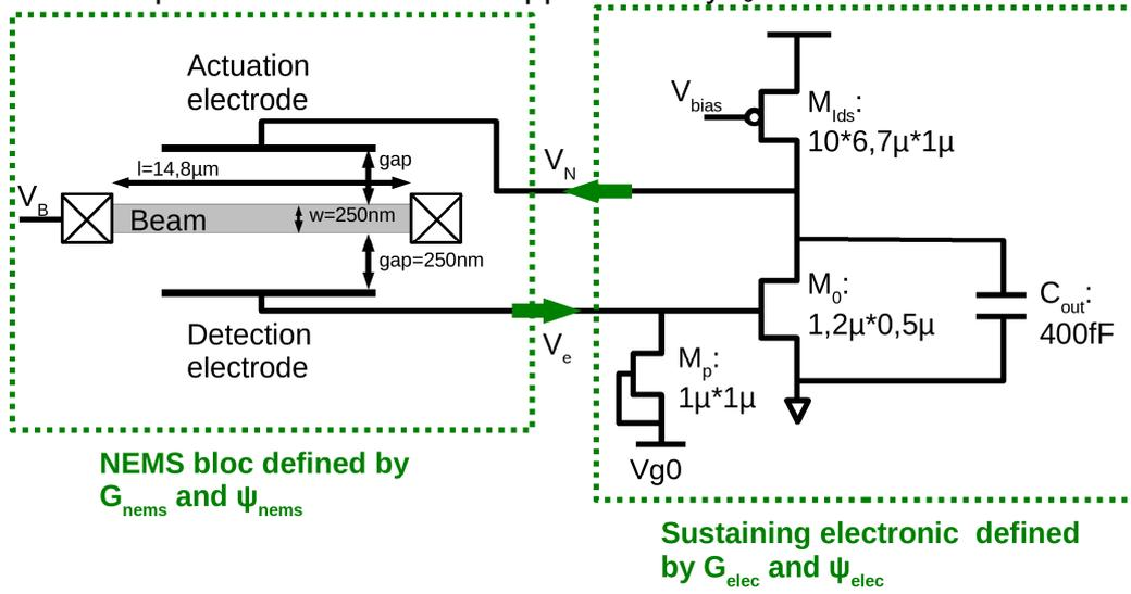
Figure 1: Oscillator schematic
