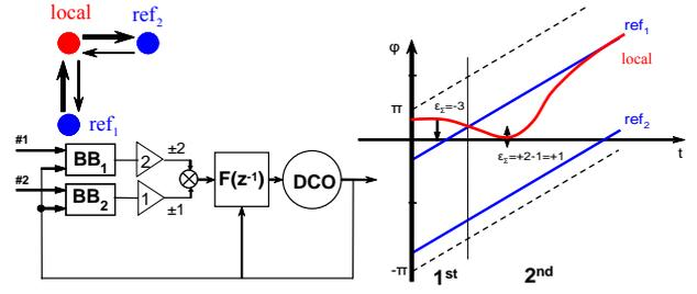
Figure 7. Node with asymmetric comparison strategy, mode-locking avoidance
