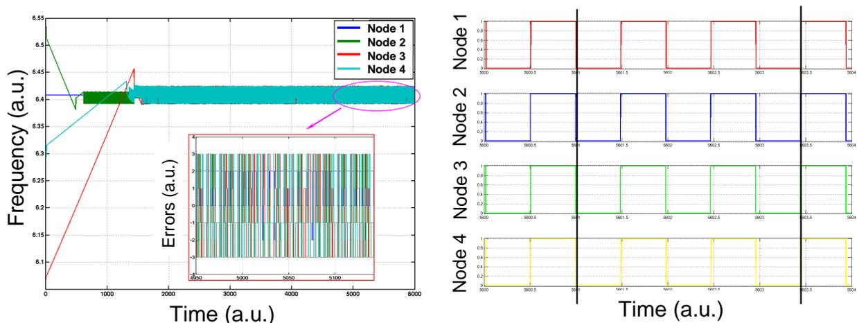
Figure 9. Simulation results on a 2x2 network with an asymmetric comparison strategy: frequency of the nodes and a zoom on their errors with the master clock (left), temporal signal in steady state of each generated clock (right)
