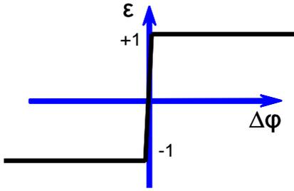
Figure 5. Bang-bang phase detector static response in phase domain
