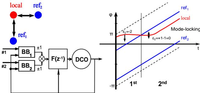
Figure 6. Node without asymmetric comparison strategy, mode-locking
