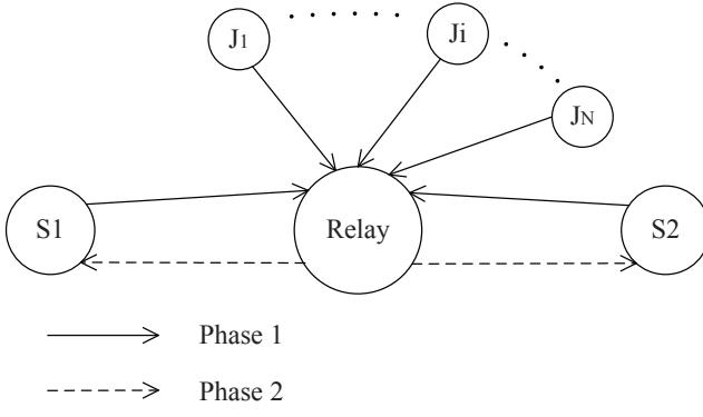
Fig. 1. System model for two-way relay communications with friendly jammers
