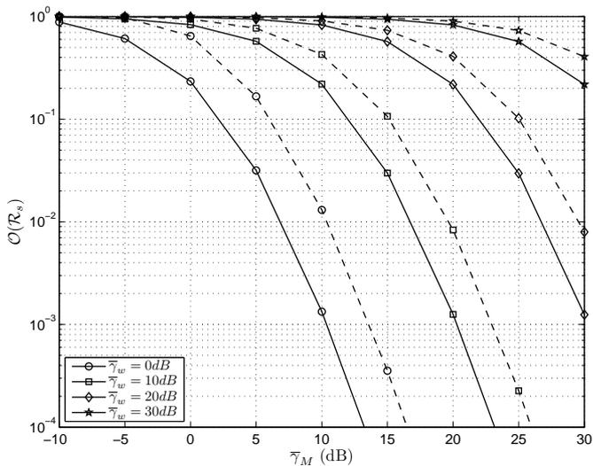
Fig. 3. Secrecy outage probability as a function of  $\bar{\gamma}_M$ , for different  $\bar{\gamma}_W$ . The solid lines and the dash lines represent, respectively,  $\mathcal{R}_s = 0.1\text{bps/s/Hz}$  and  $\mathcal{R}_s = 1\text{bps/s/Hz}$ .
