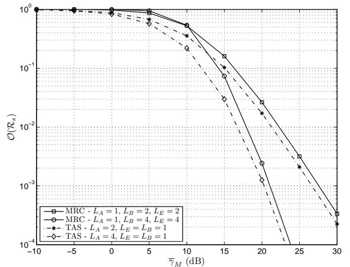
Fig. 5. Secrecy outage probability, as a function of  $\bar{\gamma}_M$ . We compare the performance between the proposed scheme (TAS) and that in [9] (MRC) when  $\bar{\gamma}_W = 10\text{dB}$  and  $\mathcal{R}_s = 0.1\text{bits/s/Hz}$ , and where  $L_B$  and  $L_E$  are the number of antennas at Bob and Eve.
