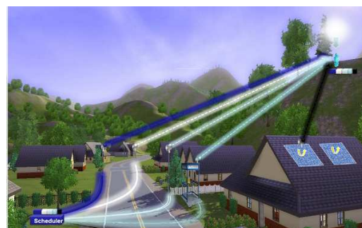
Fig. 2. The small reconfigurable base stations are plugged on an heterogeneous infrastructure (powerline, ADSL, fiber optics,..) to serve the various users in the network. A scheduler splits the packets on the different routes of the wired network.
