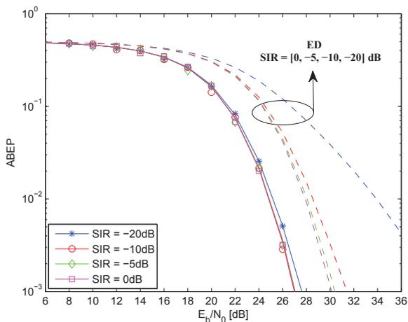
Fig. 5. ABEP of  $T_c$ -DTR and ED receivers. Solid lines: analytical model. Markers: Monte Carlo simulation. As far as the  $T_c$ -DTR scheme is considered, a Walsh-Hadamard code [77] with  $N_s = 64$  is considered. The ED receiver for  $N_s = 64$  is shown with dashed lines (only model).
