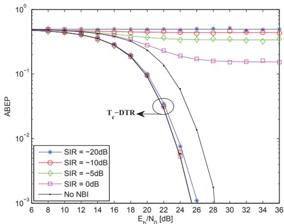
Fig. 3. ABEP of  $T_c$ -DTR and TR receivers. Solid lines: analytical model. Markers: Monte Carlo simulation. As far as the  $T_c$ -DTR scheme is considered, the optimal DS code design to meet the conditions  $C_1$  and  $C_2$  is considered. The used code is  $[-1, +1, -1, +1, \dots]$ . Parameter setup for TR: i) BPAM modulation, and ii)  $T_r = 60\text{ns}$ .
