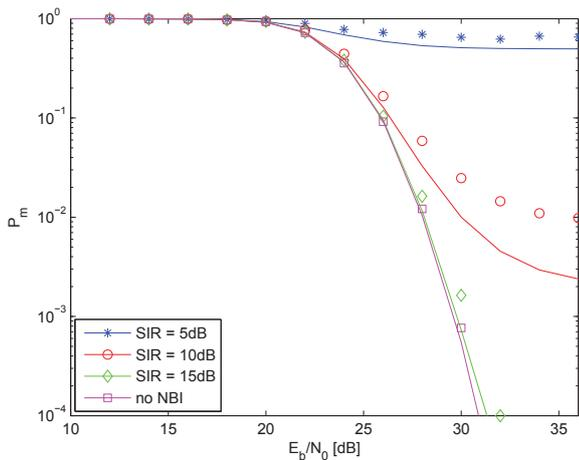
Fig. 13.  $P_m$  of the DTR receiver with 3 interferers located at  $f_{J_1} = 0.9054\text{GHz}$  (GSM band),  $f_{J_2} = 1.38105\text{GHz}$  (GNSS band), and  $f_{J_3} = 2.452\text{GHz}$  (802.11b Wi-Fi band). The receiver is optimized (on average) to reject the aggregate NBI, *i.e.*,  $T_c = 87.90\text{ns}$ .
