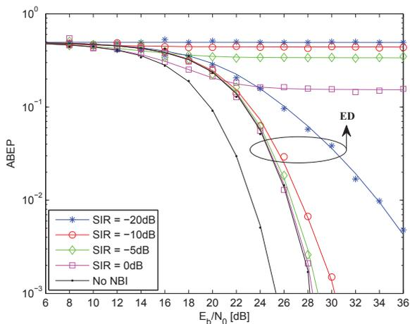
Fig. 2. ABEP of DTR and ED receivers. Solid lines: analytical model. Markers: Monte Carlo simulation. Parameter setup for DTR: i) BPAM modulation, ii)  $T_c = 60\text{ns}$ , and iii)  $T_b = N_s T_c$ . Parameter setup for ED: i) (Binary)PPM modulation, ii)  $T_c = 120\text{ns}$ , and iii) the PPM modulation shift is  $60\text{ns}$ .
