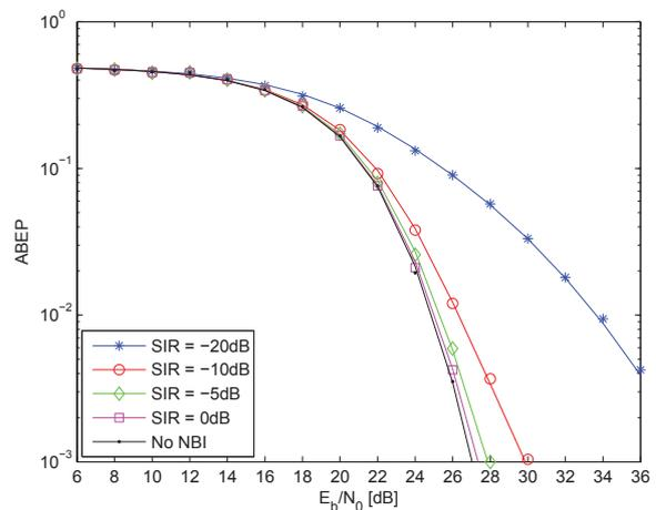
Fig. 4. ABEP of CM-TR receiver. Solid lines: analytical model. Markers: Monte Carlo simulation. Parameter setup: i) BPAM modulation, ii)  $T_c = 60\text{ns}$ , and iii)  $T_b = N_s T_c$ . Furthermore, the multiplexing codes are assumed to satisfy the condition in [12, Eq. (8)].
