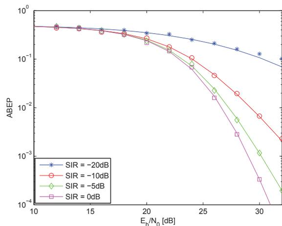
Fig. 11. ABEP of the ED receiver with 3 interferers located at  $f_{J_1} = 0.9054\text{GHz}$  (GSM band),  $f_{J_2} = 1.38105\text{GHz}$  (GNSS band), and  $f_{J_3} = 2.452\text{GHz}$  (802.11b Wi-Fi band).  $T_c = 60\text{ns}$
