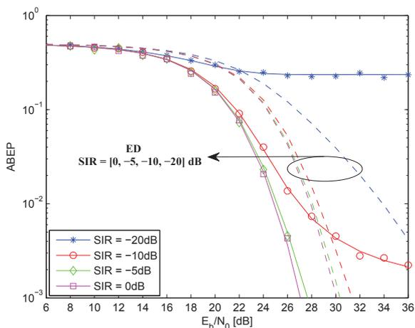
Fig. 6. ABEP of  $T_c$ -DTR and ED receivers. Solid lines: analytical model. Markers: Monte Carlo simulation. As far as the  $T_c$ -DTR scheme is considered, a ML code [77] with  $N_s = 63$  is considered. The ED receiver for  $N_s = 63$  is shown with dashed lines (only model).
