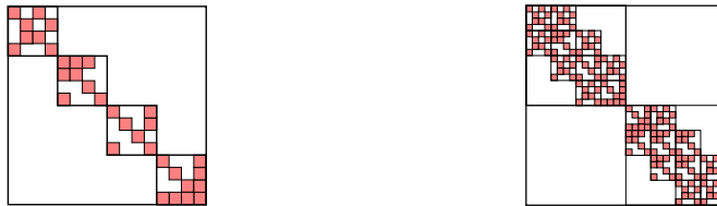
Fig. 1. Block Matrix Patterns. A block diagonal matrix pattern is represented on the left while a block diagonal matrix with tridiagonal blocks is represented on the right.
