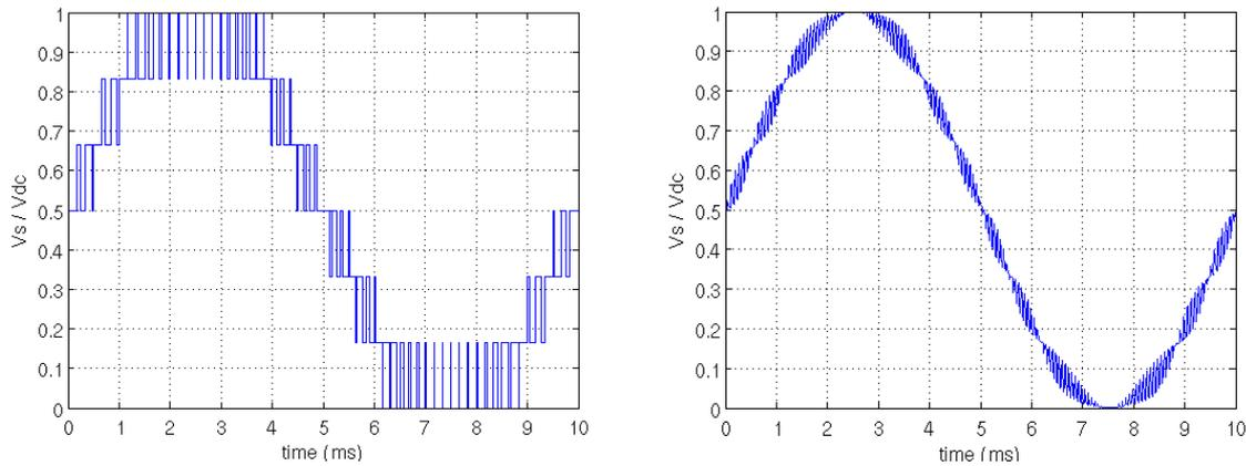
Fig. 2: Output voltage  $v_s$  of a 6 Cells Interleaved Inverter, without (2.a) and with (2.b) filtering effects
