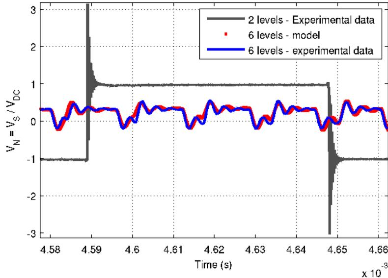
Fig. 9: Zoom on a switching period of the voltage across the load at the cable end
