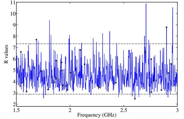
Figure 5. The maximum normalized power value  $R$  of the unloaded case are plotted as a function of frequency (solid line). Bounding values of the CI (dashed line) are taken from Fig. 1 and markers highlight the frequencies that did not pass the GoF test.
