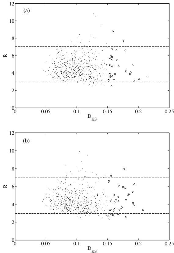
Figure 6. Scatter plot of  $R$  versus  $D_{KS}$  for (a) the unloaded scenario (b) the loaded scenario. Black-colored dots represent the cases for which the null hypothesis  $H_0$  is accepted; black circles represent the cases for which  $H_0$  is rejected. Bounding values of the CI are also reported (dashed lines).
