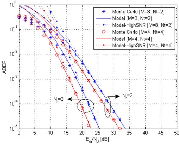
Fig. 4. ABEP of SM-QAM against  $E_m/N_0$ . Performance comparison for various sizes of signal- and spatial-constellation diagrams. Accuracy of proposed analytical frameworks for unit-power ( $\sigma_0^2 = 1$ ) i.i.d. Rayleigh fading (the rate is  $R = 4$  bpcu). The setup ( $M = 2, N_t = 8$ ) is not shown, as it overlaps with the setup ( $M = 4, N_t = 4$ ).
