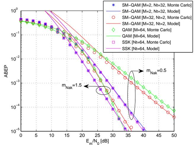
Fig. 10. ABEP against  $E_m/N_0$  over i.i.d. Nakagami- $m$  fading ( $m_{\text{Nak}} = 0.5$  and  $m_{\text{Nak}} = 1.5$ ,  $N_r = 2$ , and rate  $R = 6$  bpcu). Performance comparison and accuracy of the analytical framework for SM-QAM, QAM, and SSK.
