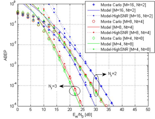
Fig. 5. ABEP of SM-PSK against  $E_m/N_0$ . Performance comparison for various sizes of signal- and spatial-constellation diagrams. Accuracy of proposed analytical frameworks for unit-power ( $\sigma_0^2 = 1$ ) i.i.d. Rayleigh fading (the rate is  $R = 5$  bpcu). The setup ( $M = 2, N_t = 16$ ) is not shown, as it overlaps with the setup ( $M = 4, N_t = 8$ ).
