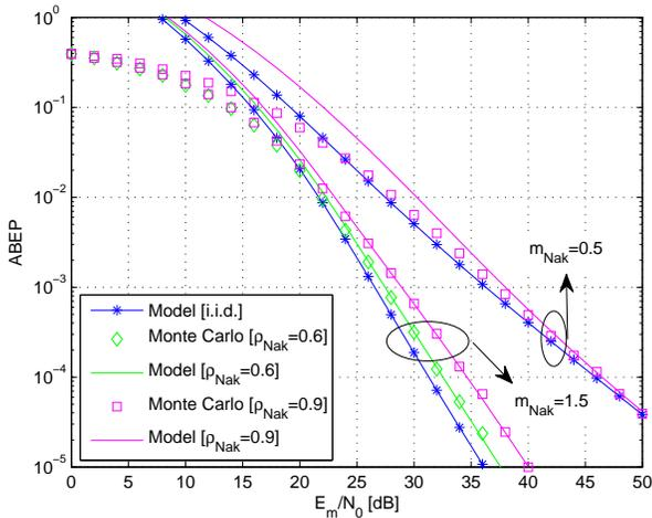
Fig. 12. ABEP of SM-QAM against  $E_m/N_0$  over correlated (at the transmitter) and identically distributed Nakagami- $m$  fading ( $m_{\text{Nak}} = 0.5$  and  $m_{\text{Nak}} = 1.5$ ,  $N_r = 2$ , and rate  $R = 6$  bpcu). Performance comparison and accuracy of the analytical framework for  $M = 32$  and  $N_t = 2$ .
