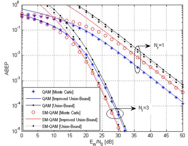
Fig. 2. ABEP of QAM ( $M^{\text{QAM}} = 64$ ) and SM-QAM ( $M = 32$ ,  $N_t = 2$ ) against  $E_m/N_0$ . Accuracy of proposed analytical framework (denoted by “improved union-bound” in the legend) and conventional union-bound (denoted by “union-bound” in the legend) for unit-power ( $\sigma_0^2 = 1$ ) i.i.d. Rayleigh fading (the rate is  $R = 6$ bpcu).
