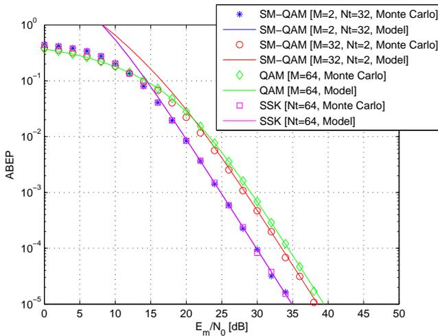
Fig. 9. ABEP against  $E_m/N_0$  over i.i.d. Nakagami- $m$  fading ( $m_{\text{Nak}} = 1.0$ , i.e., Rayleigh,  $N_r = 2$ , and rate  $R = 6$  bpcu). Performance comparison and accuracy of the analytical framework for SM-QAM, QAM, and SSK.
