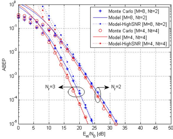
Fig. 3. ABEP of SM-PSK against  $E_m/N_0$ . Performance comparison for various sizes of signal- and spatial-constellation diagrams. Accuracy of proposed analytical frameworks for unit-power ( $\sigma_0^2 = 1$ ) i.i.d. Rayleigh fading (the rate is  $R = 4$  bpcu). The setup ( $M = 2, N_t = 8$ ) is not shown, as it overlaps with the setup ( $M = 4, N_t = 4$ ).
