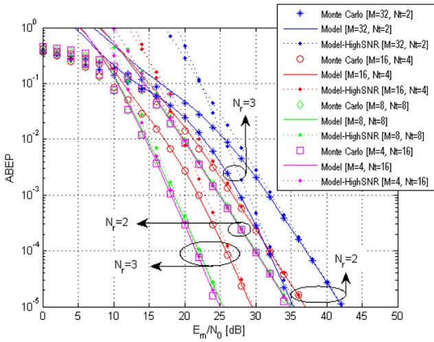
Fig. 7. ABEP of SM-PSK against  $E_m/N_0$ . Performance comparison for various sizes of signal- and spatial-constellation diagrams. Accuracy of proposed analytical frameworks for unit-power ( $\sigma_0^2 = 1$ ) i.i.d. Rayleigh fading (the rate is  $R = 6$  bpcu). The setup ( $M = 2$ ,  $N_t = 32$ ) is not shown, as it overlaps with the setup ( $M = 4$ ,  $N_t = 16$ ).
