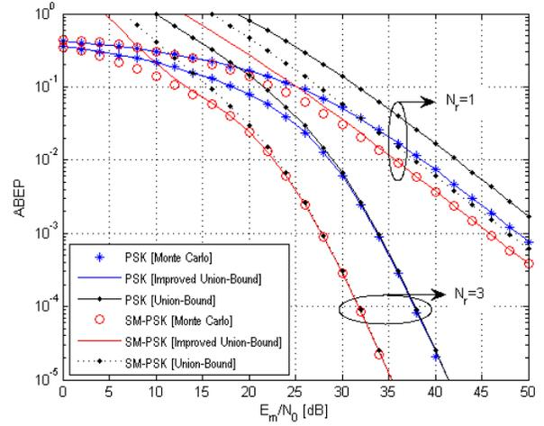
Fig. 1. ABEP of PSK ( $M^{\text{PSK}} = 64$ ) and SM-PSK ( $M = 32$ ,  $N_t = 2$ ) against  $E_m/N_0$ . Accuracy of proposed analytical framework (denoted by “improved union-bound” in the legend) and conventional union-bound (denoted by “union-bound” in the legend) for unit-power ( $\sigma_0^2 = 1$ ) i.i.d. Rayleigh fading (the rate is  $R = 6$ bpcu).
