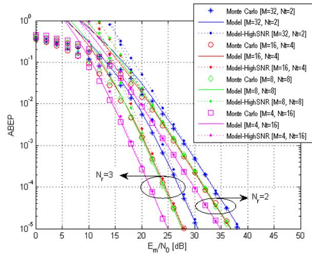
Fig. 8. ABEP of SM-QAM against  $E_m/N_0$ . Performance comparison for various sizes of signal- and spatial-constellation diagrams. Accuracy of proposed analytical frameworks for unit-power ( $\sigma_0^2 = 1$ ) i.i.d. Rayleigh fading (the rate is  $R = 6$  bpcu). The setup ( $M = 2$ ,  $N_t = 32$ ) is not shown, as it overlaps with the setup ( $M = 4$ ,  $N_t = 16$ ).
