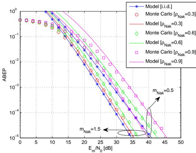
Fig. 11. ABEP of SM-QAM against  $E_m/N_0$  over correlated (at the transmitter) and identically distributed Nakagami- $m$  fading ( $m_{\text{Nak}} = 0.5$  and  $m_{\text{Nak}} = 1.5$ ,  $N_r = 2$ , and rate  $R = 6$  bpcu). Performance comparison and accuracy of the analytical framework for  $M = 2$  and  $N_t = 32$ .
