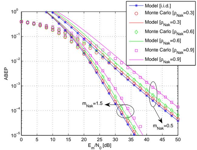
Fig. 14. ABEP of SM-QAM against  $E_m/N_0$  over correlated (at the receiver) and identically distributed Nakagami- $m$  fading ( $m_{\text{Nak}} = 0.5$  and  $m_{\text{Nak}} = 1.5$ ,  $N_r = 2$ , and rate  $R = 6$  bpcu). Performance comparison and accuracy of the analytical framework for  $M = 32$  and  $N_t = 2$ .
