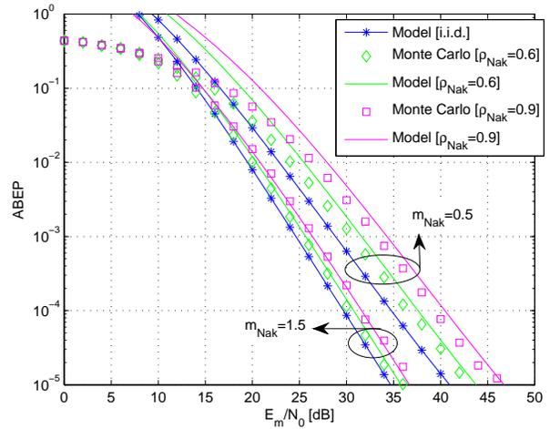
Fig. 13. ABEP of SM-QAM against  $E_m/N_0$  over correlated (at the receiver) and identically distributed Nakagami- $m$  fading ( $m_{\text{Nak}} = 0.5$  and  $m_{\text{Nak}} = 1.5$ ,  $N_r = 2$ , and rate  $R = 6$  bpcu). Performance comparison and accuracy of the analytical framework for  $M = 2$  and  $N_t = 32$ .
