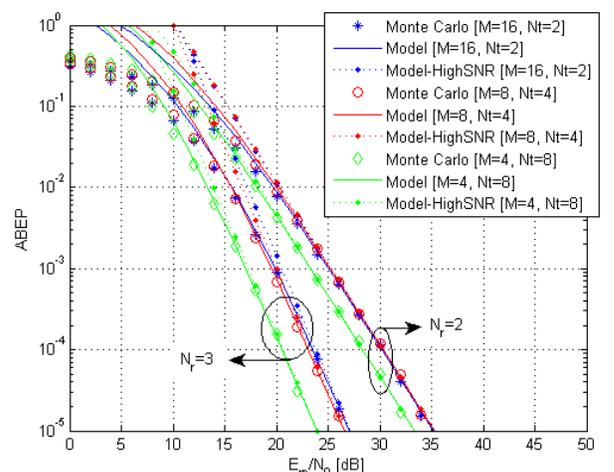
Fig. 6. ABEP of SM-QAM against  $E_m/N_0$ . Performance comparison for various sizes of signal- and spatial-constellation diagrams. Accuracy of proposed analytical frameworks for unit-power ( $\sigma_0^2 = 1$ ) i.i.d. Rayleigh fading (the rate is  $R = 5$  bpcu). The setup ( $M = 2, N_t = 16$ ) is not shown, as it overlaps with the setup ( $M = 4, N_t = 8$ ).
