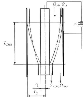
Fig. 2. Schematic diagram of a cylindrical DMA column
