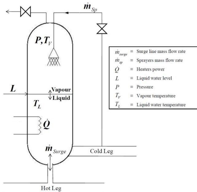
Figure 9 Simplified model of a pressurizer
