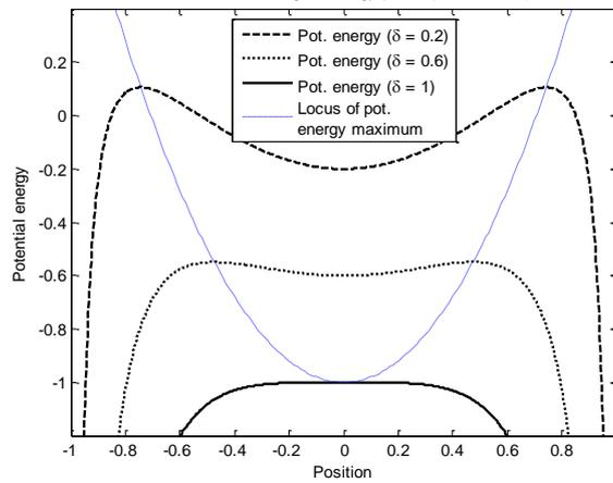
Figure 2. Potential energy (arbitrary units) vs. normalized position for a parallel-plate structure. For values of  $\delta < 1$ , the central position is stable and there exist two symmetric statically unstable equilibrium positions. For  $\delta \geq 1$ , the central position is the only equilibrium position and it is unstable.
