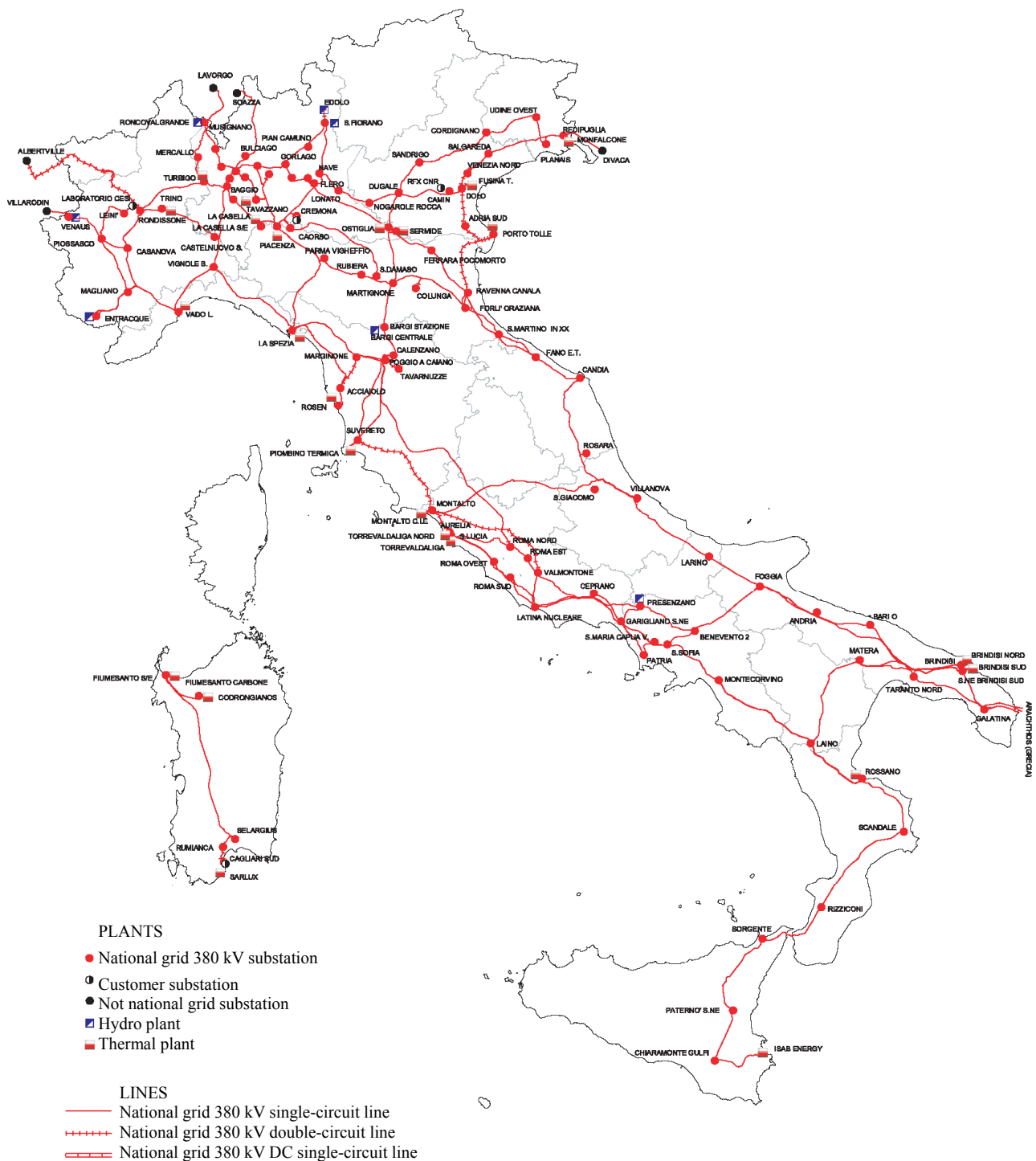
Figure 1. The 380 kV Italian power transmission network.
