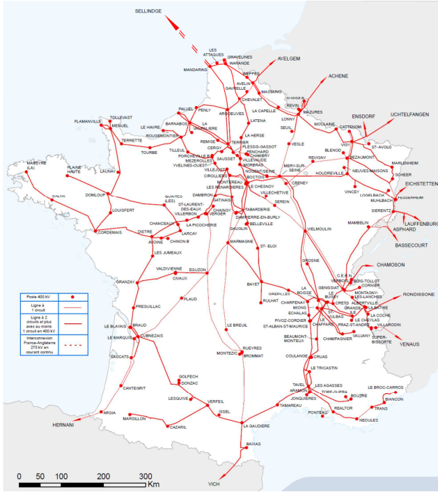
Figure 1. The 400kV French power transmission network
