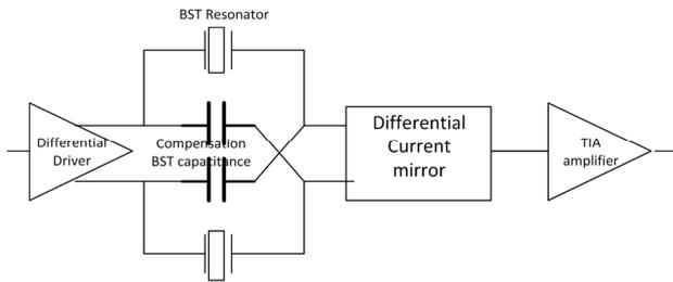
Figure 3. Parasitic capacitance compensation circuit.
