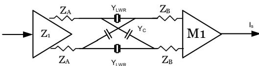
Figure 4. Model of the resonator
