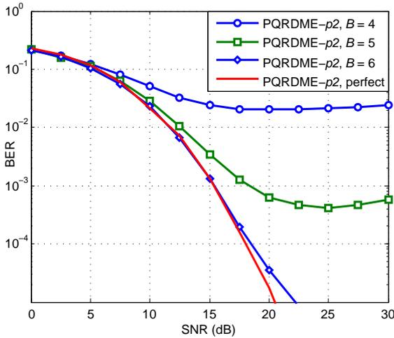
**Fig. 10** BER performance of the proposed PQRDME- $p2$  for  $M_G = T = 3$  and  $K = 8$  with imperfect CSI at the transmitter. The phase of each channel coefficient is uniformly quantized and represented by  $B$  bits.
