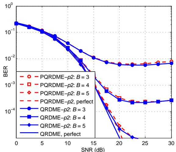
**Fig. 9** BER performance of the proposed PQRDME- $p2$  for  $M_G = T = 3$  and  $K = 8$  with imperfect CSI at the transmitter. The real and imaginary parts are quantized using Lloyd-Max non-uniform quantizer, where each part is represented by  $B$  bits.
