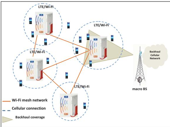
Fig. 1. Outdoor coverage network in poorly covered areas.
