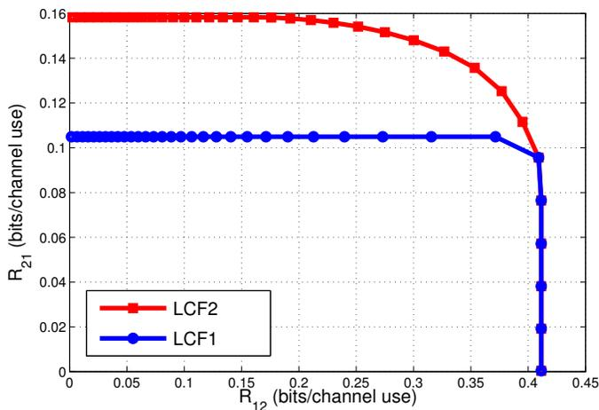
(a)  $P_1 = 10$  dB,  $P_2 = P_R = 5$  dB,  $|h_1|^2 = 2$ ,  $|h_2|^2 = 0.5$
