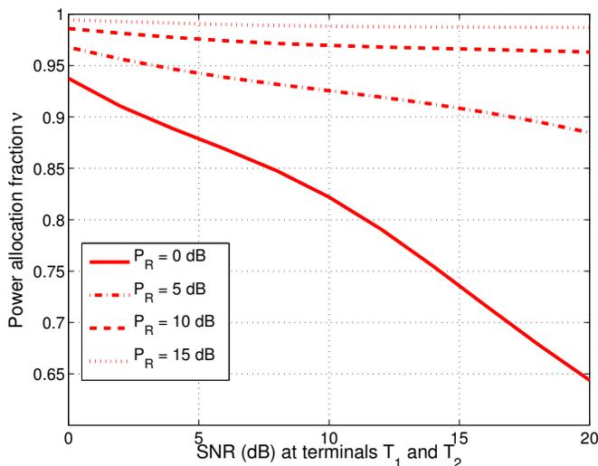
Fig. 10: Relay power allocation fraction  $\nu$  in LCF2 for different fixed relay transmit power  $P_R$  and equal SNR  $= \frac{P_1}{\sigma_R^2} = \frac{P_2}{\sigma_R^2}$  at both terminals,  $|h_1|^2 = 4$  and  $|h_2|^2 = 0.5$ .
