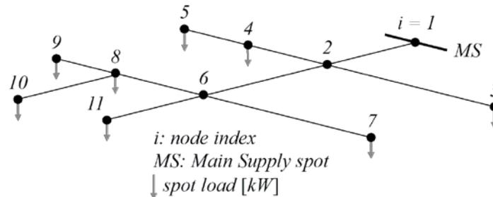
Figure 5. Radial 11-nodes distribution network
