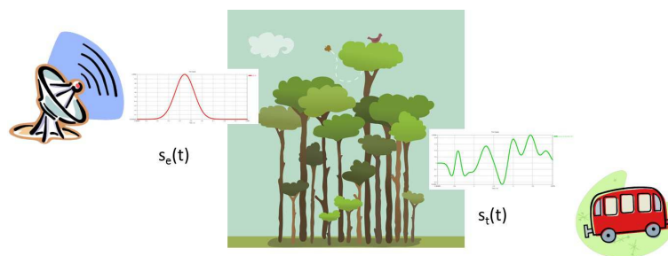
Fig. 1: A radar emits the signal s_e(t) which the forest modifies to s_t(t) before it reaches the target.
