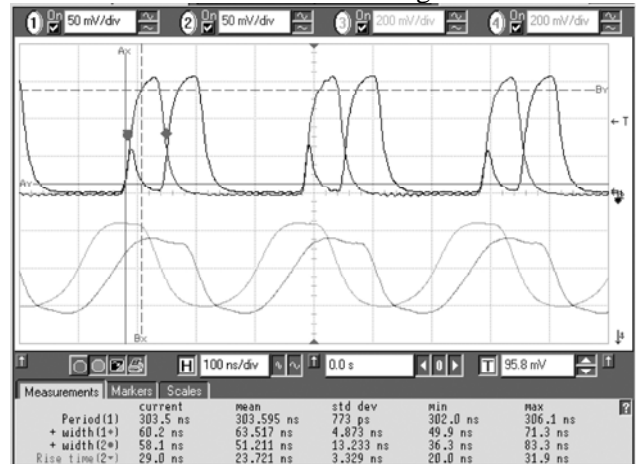
Fig. 4 – Measured feedback (top) and output (bottom) waveforms. The output waveforms are slightly distorted due to feedthrough and saturation effects. The duty cycle of the feedback waveforms is a direct measurement of the phase delay \phi .
