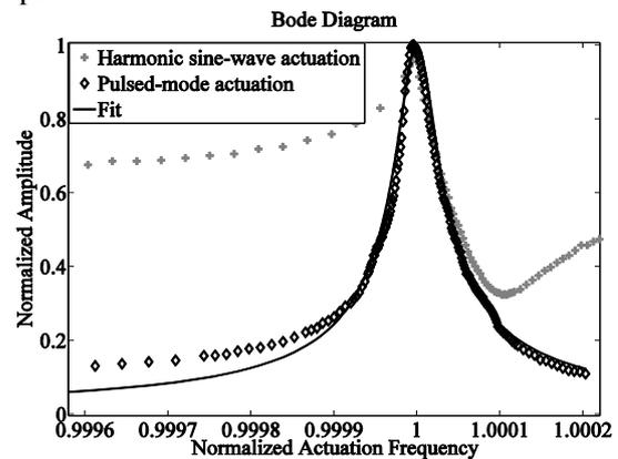
**Fig. 6:** Bode diagram obtained with harmonic sine-wave actuation (grey crosses) and pulsed-mode actuation after de-embedding (diamonds). The continuous dark line shows the curve fitted to the pulsed-mode response.
