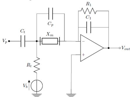
**Fig. 3:** Test circuit. The  $X_m$ -element is the resonator.  $V_b = 10V$  is the bias voltage and  $V_p$  the 2V-amplitude and 150ns-width pulses.  $C_t = 1\mu F$ ,  $R_t = 1k\Omega$ ,  $C_1 = 10pF$  and  $R_1 = 1.0M\Omega$ .  $C_p$  is the unknown parasitic capacitance.
