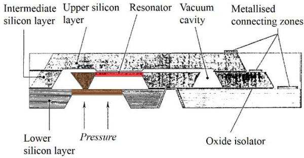
**Fig. 1:** Sensor structure (from [5]). The sensing element consists in a resonant silicon beam encapsulated in vacuum, with a massive stud bonded to a silicon diaphragm. The beam is capacitively actuated and sensed with the facing electrode.
