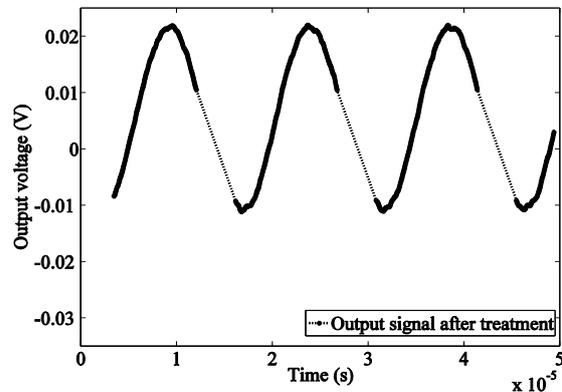
**Fig. 5:** Output voltage after “cleaning out” the pulses. This localized signal processing leaves the remaining signal completely free of feedthrough. Knowing the excitation frequency, it is simple to fit a sine wave to the remaining signal and extract its amplitude.
