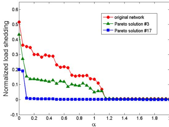
**Figure 4. Cascading vulnerability (normalized load shedding) evaluated by the OPA model for the three chosen networks over a range of network tolerance values  $\alpha$ .**
