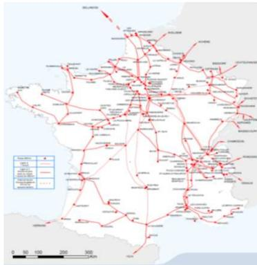
Figure 1. The 400kV French power transmission network
