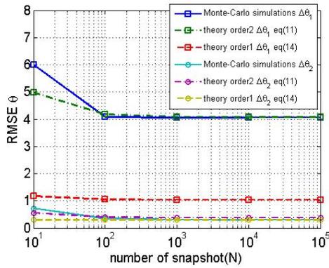
Figure 2: RMSE of DOA estimation error of  $\theta_1$  and  $\theta_2$  vs. number of snapshots (N) (2 sources with Uniform angular dispersion,  $\Delta_0 = 10^\circ$ ,  $\Delta = 15^\circ$ ,  $\theta_1 = 21^\circ$ ,  $\theta_2 = 39^\circ$ )
