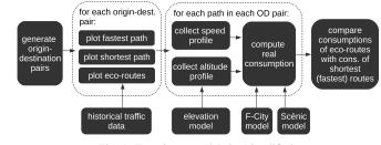
Fig. 1: Experiment toolchain (simplified)
