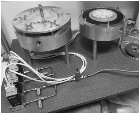
Figure 5: Cembureau device for permeability measurement in laboratory
