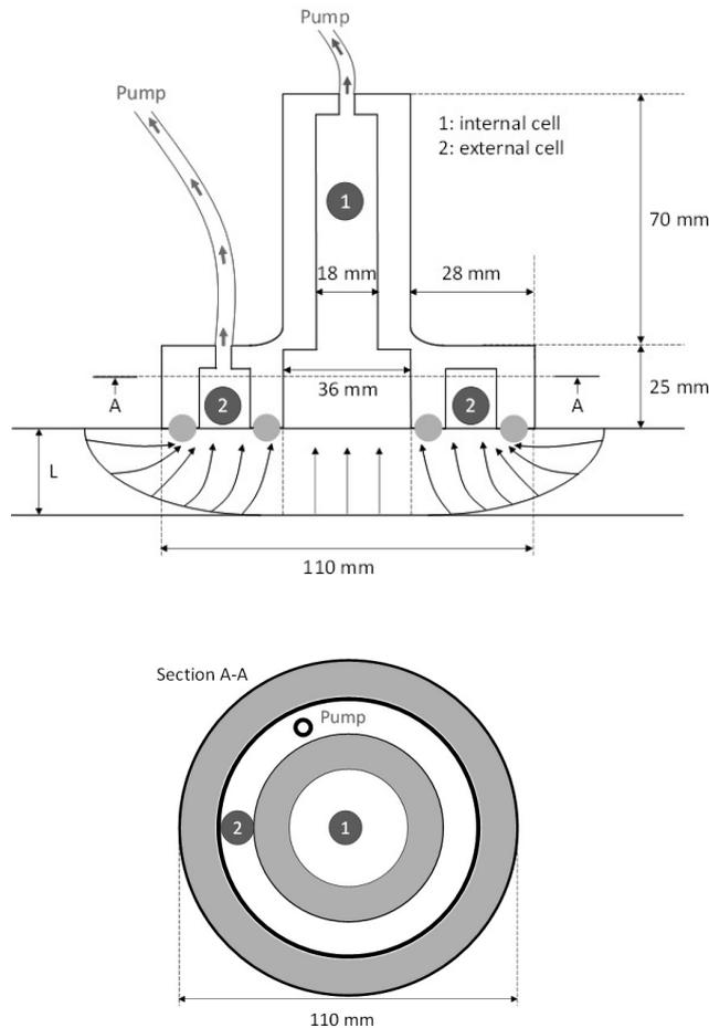
Figure 2: Pictorial representation of Torrent device for permeability measurement
