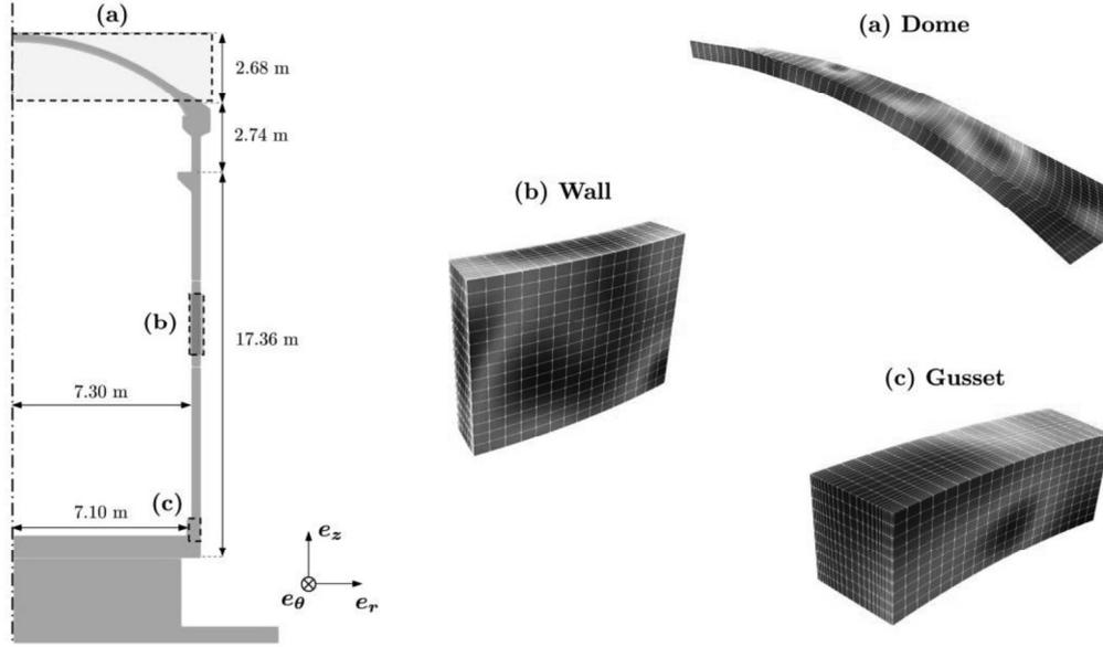
Figure 15: 2D view of the VeRCoRs mock-up (left) and some realizations of the intrinsic permeability random field on meshes of three Representative Structural Volumes (RSV) of the mock-up (right).
