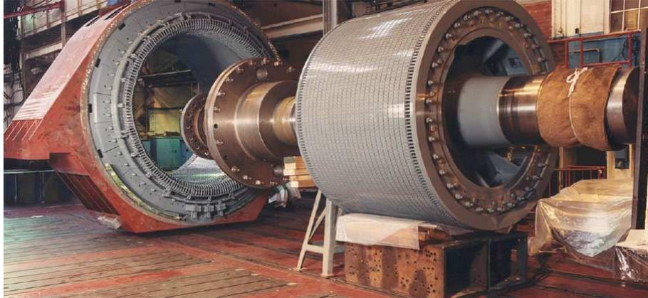
Figure 1.12 : Machine asynchrone de 4.7 MW, 45tr/mn [30]
